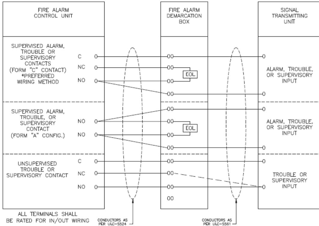
Figure 1 – Demarcation between fire alarm control unit and signal transmitting unit at the protected premises
